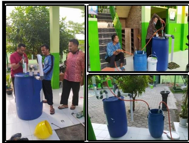
**Gambar 20.** Biodigester Gas Metan Portable
